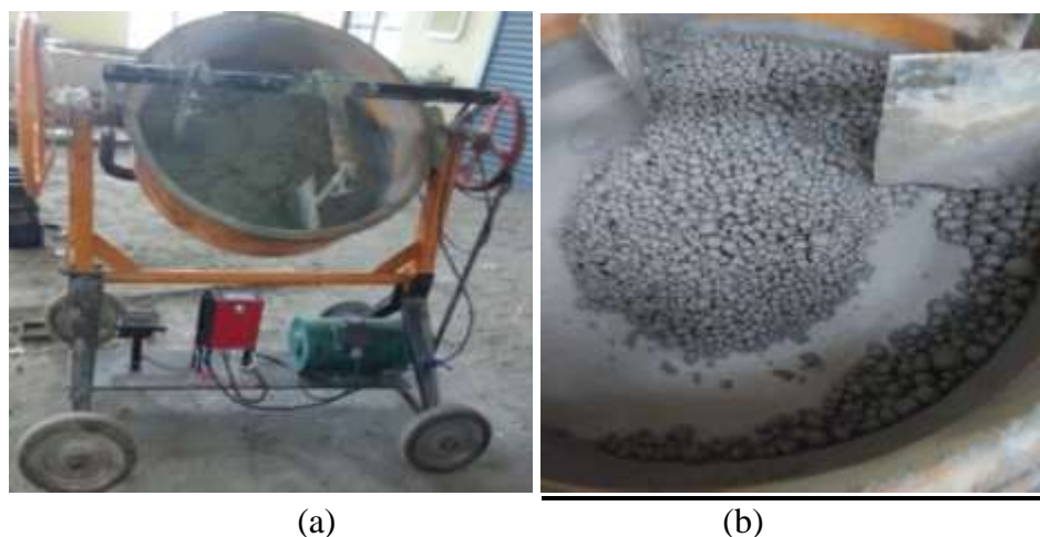
Fig. 6. Fly Ash Aggregates, (a) Pelletizer Machine, (b) Palletised Aggregates.
