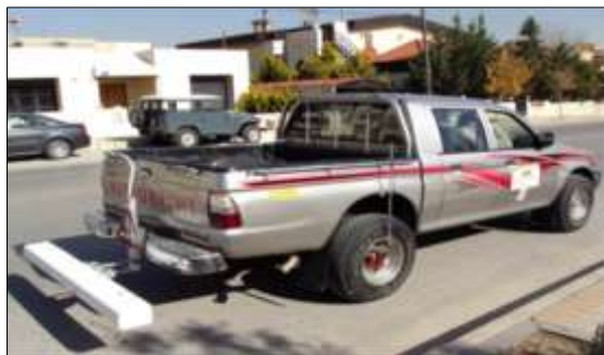
Fig. 1: Australian Road Research Board (ARRB) Laser Profiler Technology.
