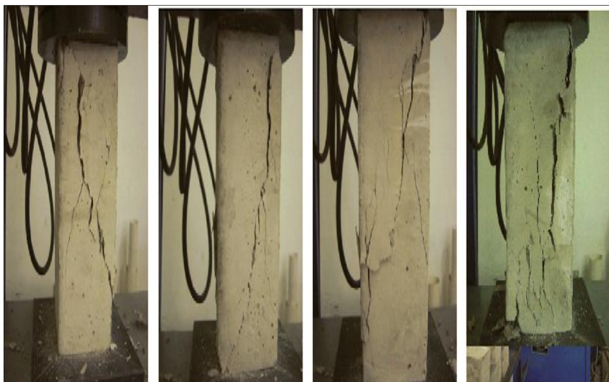
Fig. 5(b): Failure Process of Recycled Aggregate Concrete Prism [26] .
