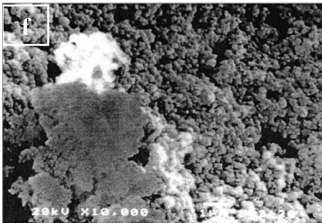
Fig. 6(f): Surface Treated RA in Silica Fume Solution [2] .
