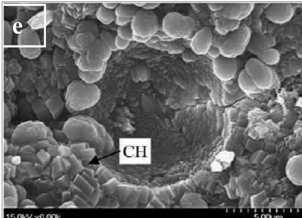
Fig. 6(e): Surface Microstructure of RA with Fly Ash [2] .
